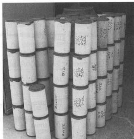
Standard capped cylinders ready for testing.
