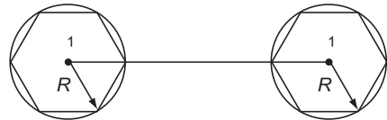
Fig. 4.14 Frequency reuse ratio q = D^2 / R^2
