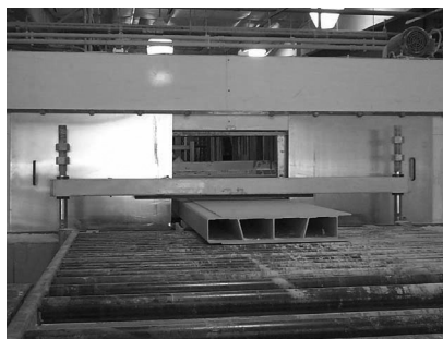
FIGURE 16.8 Pultruded hollow core FRP bridge deck. (From Godwin, G. et al., Proceeding of 3rd International Conference on Composites in Infrastructure (ICCI'02) , Omipress (CD-ROM), Paper 036, p. 12, 2002. With permission.)
