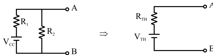
Fig.7 Potential divider circuit and its Thevenin's equivalent circuit.
