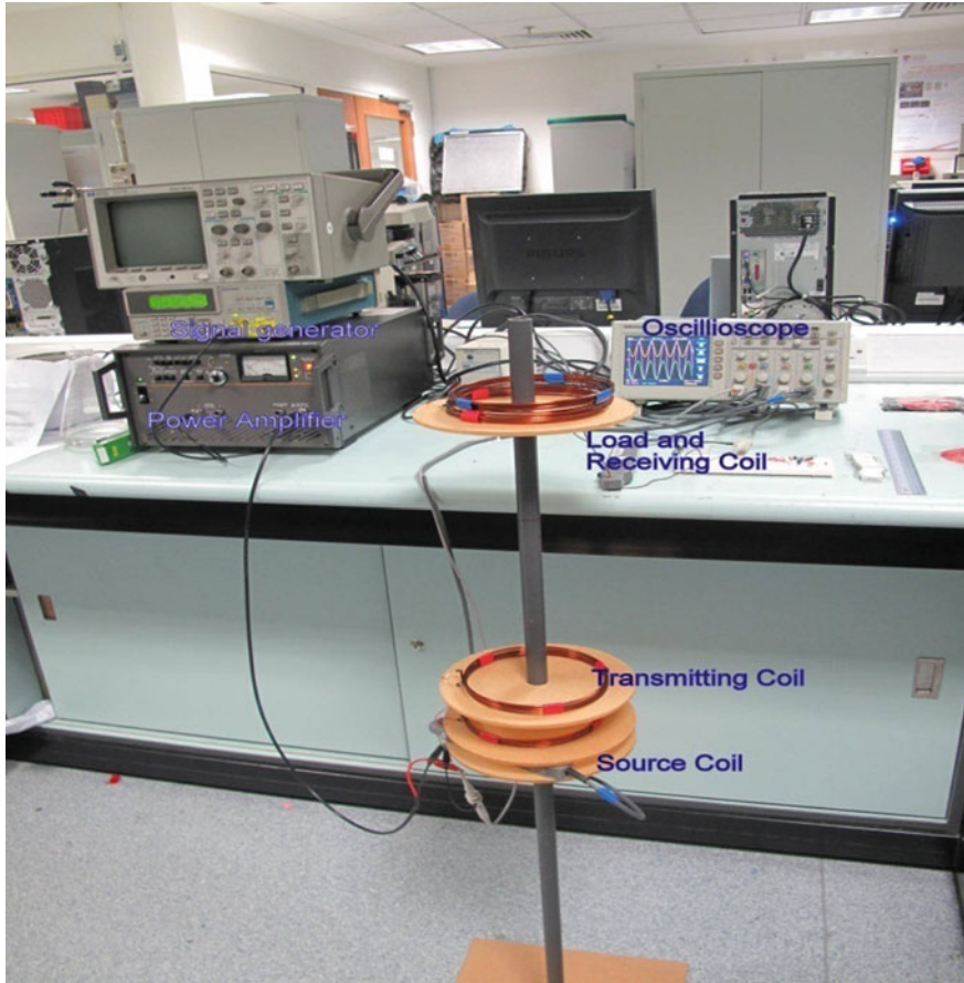
Fig. 1. Experiment setup of wireless power transfer system
