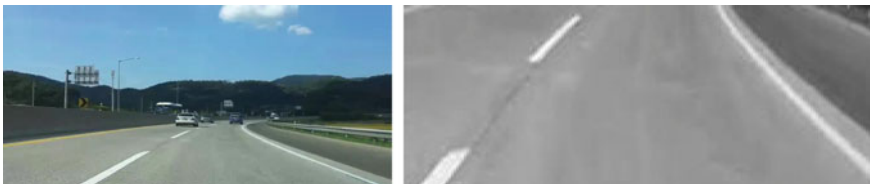
Fig. 2. (Left) Frame 6 from original video (right) Same frame after ROI selection and grayscale conversion
